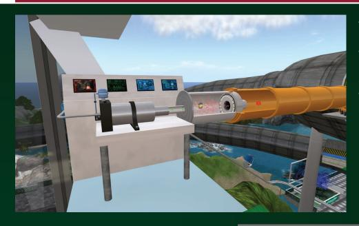
The linear accelerator is the first stage of a typical DOE accelerator. Protons begin their acceleration here at a third of their final speed.
