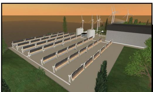
The SL representation of Enel's Archimede project includes solar panels that rotate with the SL sun. In real life these panels concentrate solar radiation on pipes containing an auxiliary fluid. The heat raises the temperature of this fluid, storing the heat for use any time of the day or during any weather conditions.
